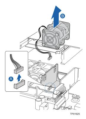
Figure 39. Removing a System Fan Module
